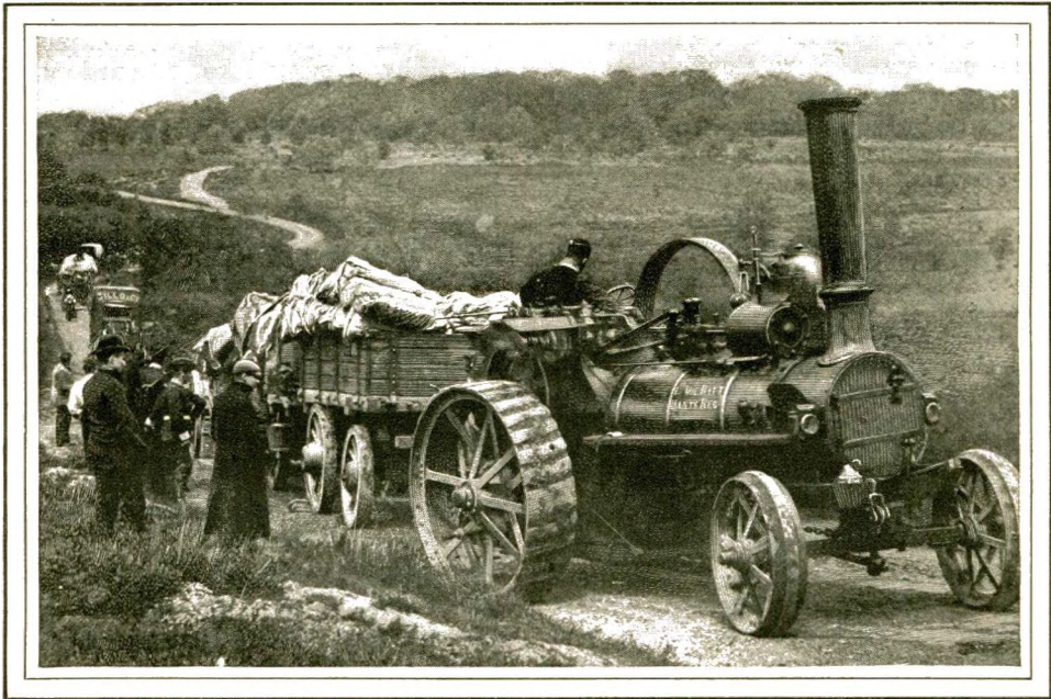
ANOTHER MODERN FORM OF THE TRACTION ENGINE—AN ENGLISH MILITARY MACHINE USED IN SOUTH AFRICA FOR MOVING ARMY SUPPLIES.
